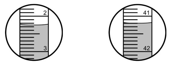
(a) In the table below. record the initial and final buret readings and the calculated value for the volume of 0.725 *M* KOH(*aq*) required to reach the end point.
